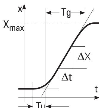
$V_{max} = \frac{X_{max}}{T_g} = \frac{\Delta x}{\Delta t}$
