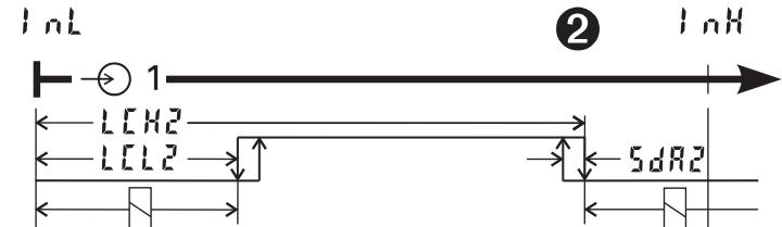
**Function of relative limit contacts LC1 / LC2 (e.g. for LC1, n.c. contact ③, n.o. contact ④)**
