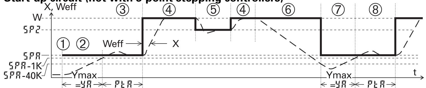
After switching on mains (1) with  $X < SPR < W$ , the process value is controlled towards set-point  $SPR$  (2),  $Y_{max} = Y_R$ . One degree below, holding time  $Pt_R$  starts (3). At holding time end, the process is lined out at set-point  $W$  (4). If switched to 2nd set-point,  $SP2$  will be valid (5). If a disturbance (6) causes the process value to drop more than 40 degrees below set-point  $SPR$ , the procedure re-starts (7) (8). **W2** blinks with running procedure.
