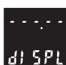
Parameter **Po int** determines the number of digits behind the decimal point in the display (0...4)., when the output value of **Func 2** is displayed (normal condition) see also p. 9, switch **L E - d i s**.
